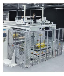
For transportation of the shaft and the bobbin in and out of the winding station the winder is equipped with a portal robot. To withdraw the bobbin from the shaft, one shaft end is fixed in a clamping device and the bobbin is withdrawn from the shaft by a moveable lifting trolley. From the trolley the bobbin can be picked up or tilted-off onto a pallet or a conveyor band.
