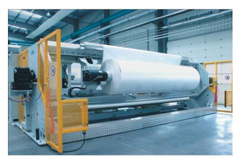
The SML turret unwinder family consists of two different types of unwinders. The PowerFlex types are designed for extra wide applications and high speeds up to 600 m/min. Due to the massive construction they can absorb vibrations very effectively. The EcoFlex unwinders give you a maximum of flexibility at a reasonable price level and speeds up to 320 m/min.
