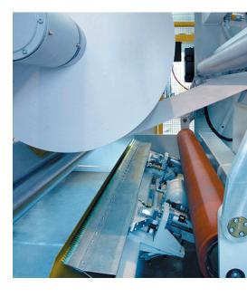
A maximum unwinding diameter of 1500 mm helps you to enlarge roll change sequences and to minimize roll loading activities.
